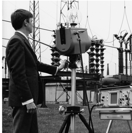
Figure 18.2 1969: ThermoVision Model 661. The camera weighed approximately 25 kg (55 lb.), the oscilloscope 20 kg (44 lb.), and the tripod 15 kg (33 lb.). The operator also needed a 220 VAC generator set, and a 10 L (2.6 US gallon) jar with liquid nitrogen. To the left of the oscilloscope the Polaroid attachment (6 kg/13 lb.) can be seen.
