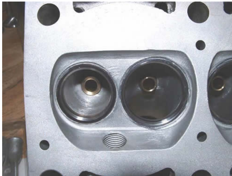
850/A112 Combustion Chamber – Note that the chamber is not yet completely finished.
