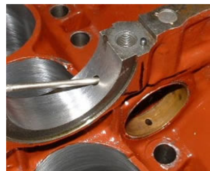
This is the 3/16th hole going to the bottom of the main cap hole from the center main.
