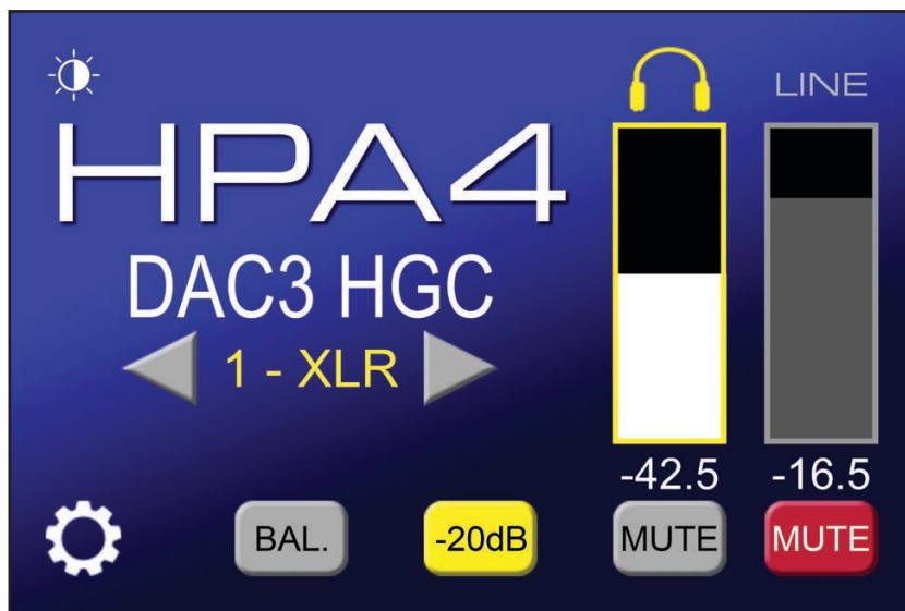
Photo 3: The attractive touchscreen display controls most of the functions of the HPA4. Channel balance can be separately adjusted for the headphone and line output groups. The gear symbol in the lower right selects the Settings menu. Volume can be individually trimmed for each of the four inputs, and the user can give each input a custom name.
