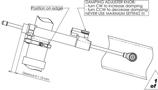
$\langle A \rangle (7) M8x35$  $\langle C \rangle$ (11)Clamp bolt M6-(6)Clamp Type 1 (5)O-ring (4)Spacer Type 1 3 M8 Hole, furthest from forkleg (8) Damper-(B)(2) M5 Clamp bolts (2x) (1) Fork bracket  $\emptyset$  52 Lower triple clamp  $\langle A \rangle (10) M8 \times 25$ (9) O-ring Standard M8 mounting hole Left frame beam  $\langle \mathsf{A}
