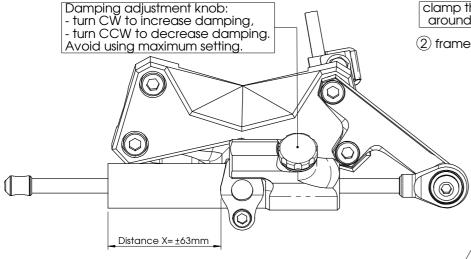
M8x40 (9) (B) -Fork bracket (8) (7) M6x25 low head  $\langle \overline{C} \rangle$  (14) Clamp bolt -M8x35 (10) (B) -Damper \$75 (11) -O-ring (12) -Spacer type 1 (13) (6) Clamp Type3 0 (5) O-ring original handlebar clamp (4) Washer M6 Ø 12 (3) M6x45 (1) frame bracket p.1 clamp the brackets around the frame (2) frame bracket p.2 loosen the brake-line clamp and bolt for more clearance during fitment
