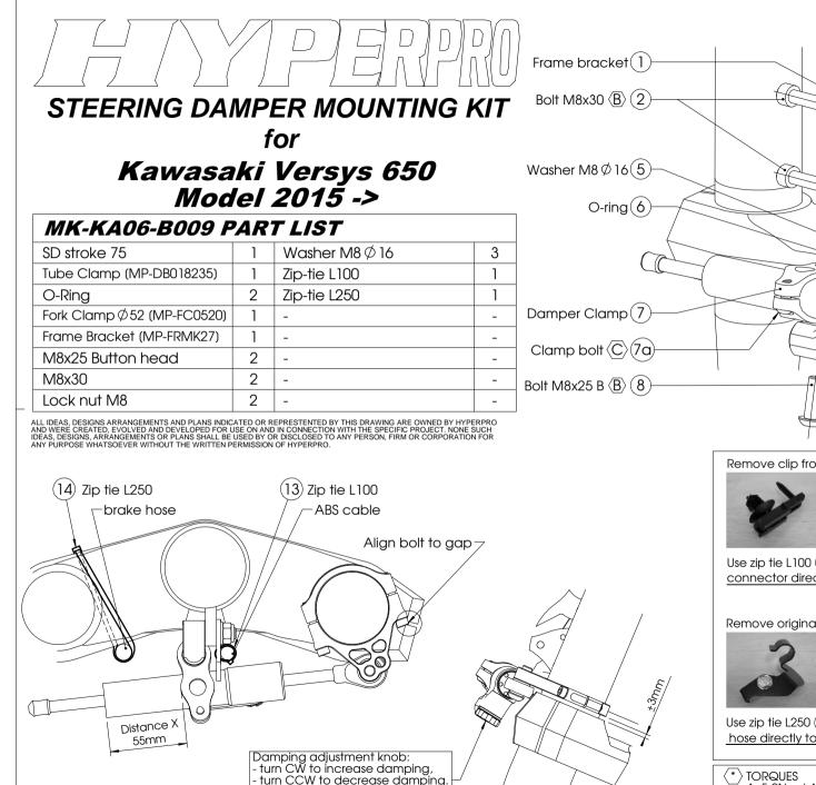
Riding direction (3) Washer M8  $\emptyset$  16  $(4)\langle B\rangle$  Lock Nut M8 (9a)  $\langle D \rangle$  Clamp bolts 9 Fork Clamp (10) O-ring (11) Damper S75  $(12)\langle B \rangle$  Bolt M8x25 B
