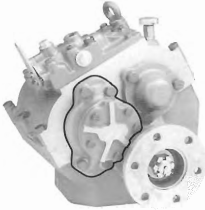
Fig. 4 Pump mounting position anti-clockwise engines
