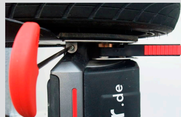
Fit rear screw of SEGautostand first
