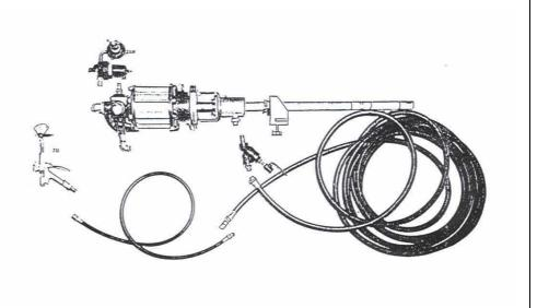
The small overall dimensions and weight of the pump predict it for portable use in places where lifting facilities are not available. These heavy duty, double action, bung mounted material pumps (pump ratio 22:1, output per minute 25 ltrs, output per cycle 200cc) are designed to dispense material from 55 gallon drums. For application of **FLUID FILM Gel B** the length of the  $\frac{3}{4}$  inch material hose should usually not exceed 45 m (3 lengths of hoses).
