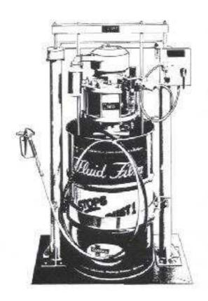
WIWA-Airless Superstar 45000 (pump ratio 46:1, output per minute 45 ltrs, output per cycle 360cc). The high-performance appliance is predicted for painting large areas and applying thick coats. It combines the high pressure ratio with a large capacity rate. With this pump a 55 US gallon (208 liter) drum may be applied in thirty-five minutes, depending upon the ease of availability of the surface to be coated.
